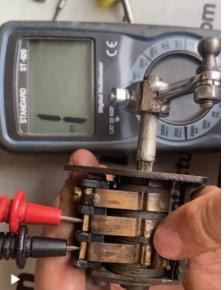
The latest discovery was the steering box mounted lighting drum switch when moved from pass lamps to P100's kept the pass lamps it. So, off came the drum switch to be fully refurbished, only to find, at some time in the car's history (pre 1962), the drum had been swapped for the one found on an SA 20 and the continued power to the pass lamps was
